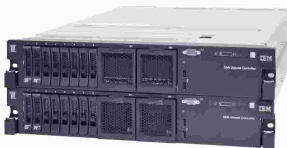
Figure 1 Front View of the two node ATRAK SVC Cluster
