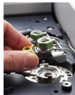
Obr. 6: Turn Top systém S/SL inletu
