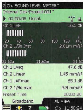
Fig. 5 Sound level meter software display showing 2-channel measurement. Channel 1 is noise, channel 2 is vibration in engineering units
