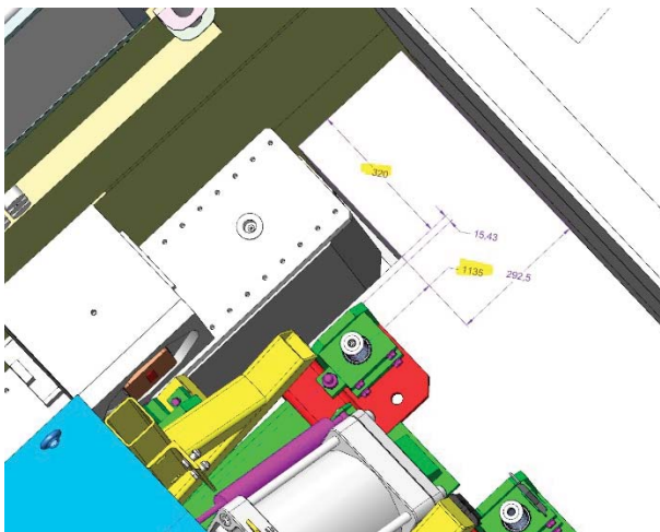
Figure 4. In red: proposed modification of support pad for fixing the shutter on the floor. The purpose is to avoid interference with the cut-out in the floor on the to-left side of the figure.
