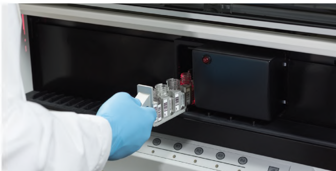
Onboard barcode reader allows real-time reagent management.
