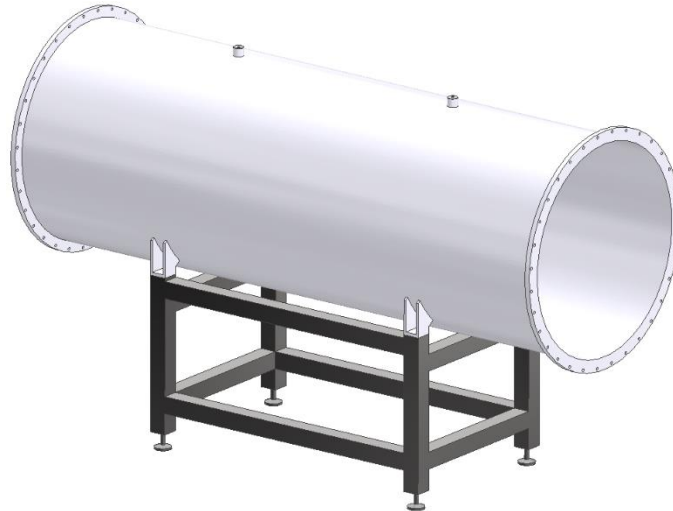
Figure 7: Conceptual design of the tubing segment supporting chassis (example of TSS1). The mounting plates on the top of the chassis shall be equipped with adjustment bolts making possible fine-tuning of the position / orientation of the tubing segment.
