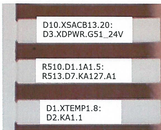
Figure 9: Example of printed labels from the printing machine Weidmüller
