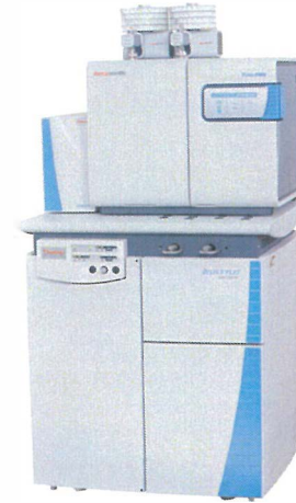
Figure 1. The Thermo Scientific EA IsoLink IRMS System.
