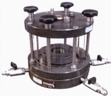
Fig 1. Low/Medium pressure cell (1 and 3MPa)
