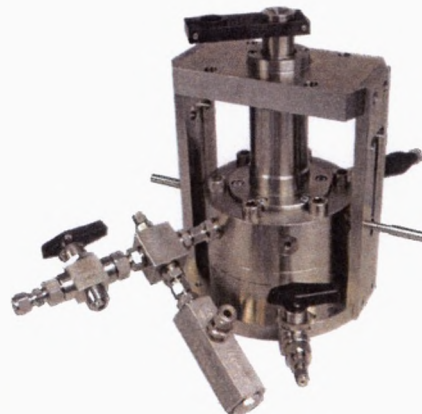
Fig 2. High pressure cell (20MPa)
