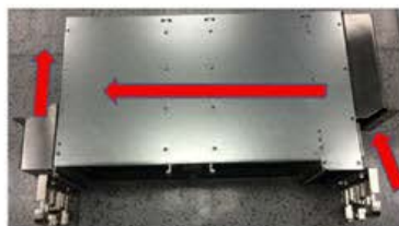
Figure 14-6 Airflow diagram - ANSI application
