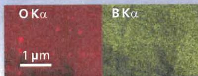
Reducing accelerating voltage from 10kV to 1.5kV allows electron image contrast to show the distribution of oxide particles. X-ray mapping under the same conditions characterises precipitates as MnOB.
