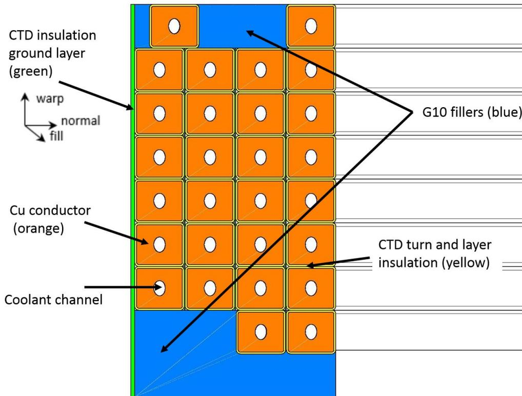
Fig. 2: Schematic cross-section of CS coil with described materials and orthotropic insulation wrap directions
