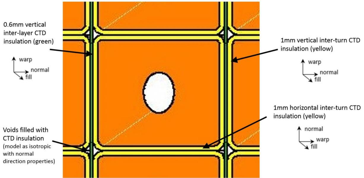
Fig. 3: Detail of inter-turn and inter-layer insulation with insulation wrap directions
