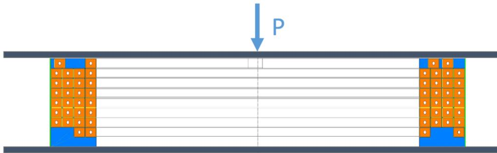
Fig. 4: Idea of the coil compression - coil placed between 2 infinitely stiff surfaces. Lower surface is fixed; upper surface is pushing on the coil with force  $P = 4 \text{ MN}$ .
