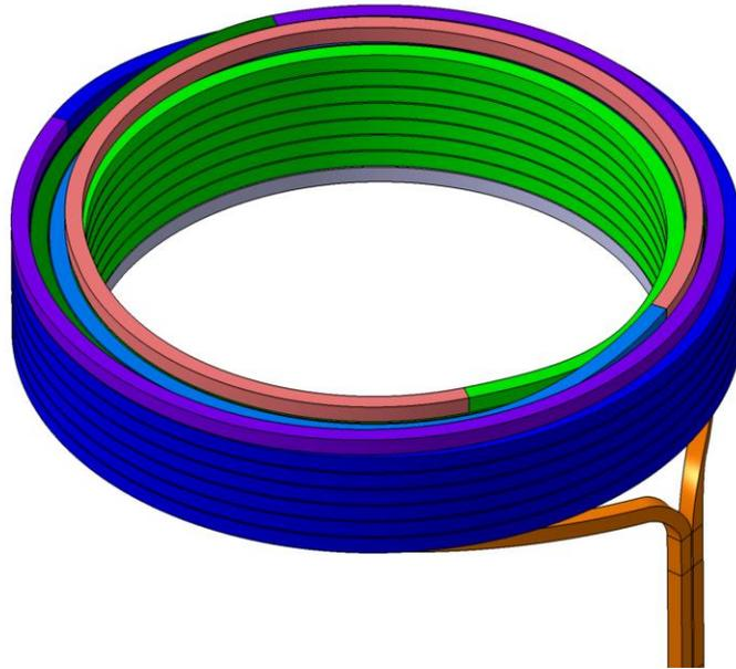
Fig.1: A model of central solenoid coil with parallel leads
