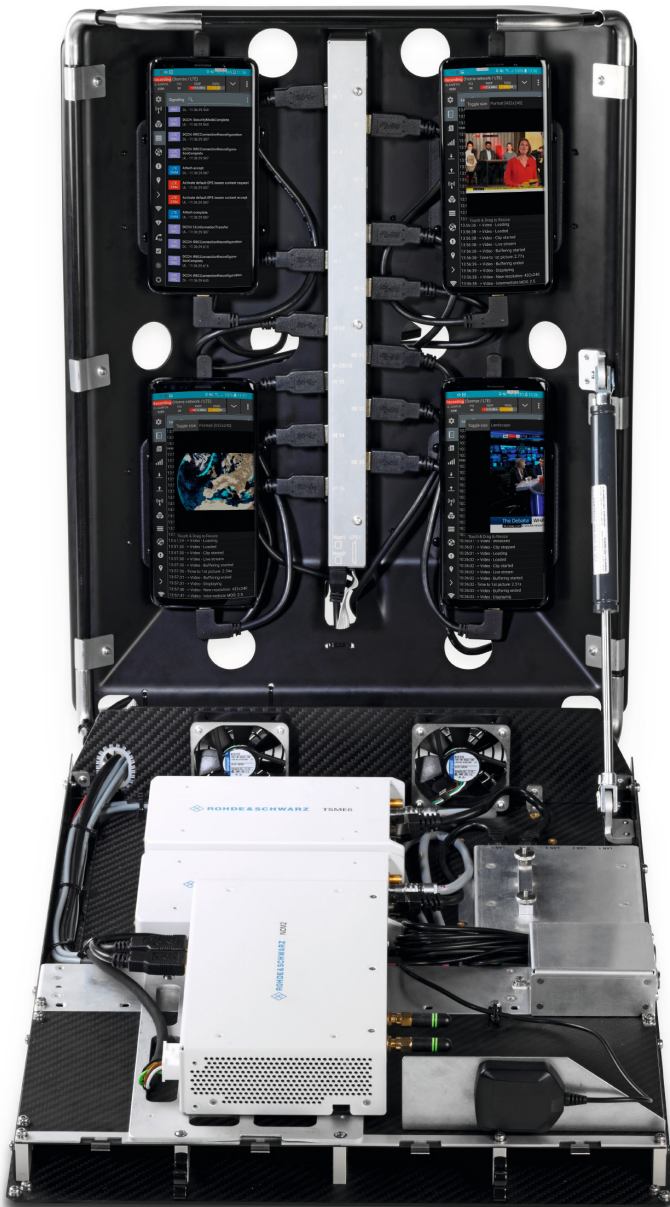
View of inside with QualiPoc, R&S®NCM2 compact integrated PC and R&S®TSM6 ultracompact drive test scanner
