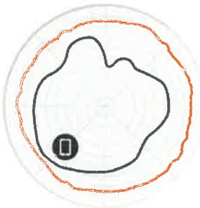
Figure 2. T300 2.4GHz Azimuth Antenna Patterns
