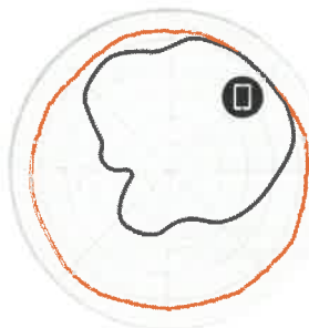
Figure 3. T300 5GHz Azimuth Antenna Patterns
