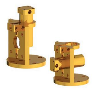
This mount provides an easily configurable way to position samples at various distances and angles with respect to the side and top optical ports. It includes a thermally damped post with standard interface bolt pattern that can be mounted vertically or horizontally to position the sample near any of the windows.
