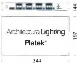
8956115 Controller LED max. 384 LED 32 DMX-RDM channels (max. 12 LEDs/channel) IN max. 60V-1080W OUT 350/500/700mA
