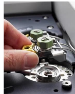
Obr. 6: Turn Top systém S/SL inletu
