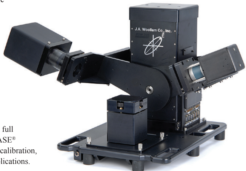
M-2000 with automated angle base, featuring a horizontal sample mount.
