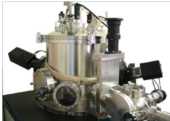
M-2000 attached to a process chamber.
