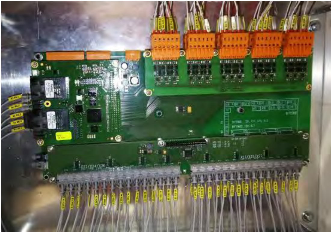
Figure 4. The smart devices used for controlling of the PS of the similar TOKAMAK developed according to order of the contractor.
