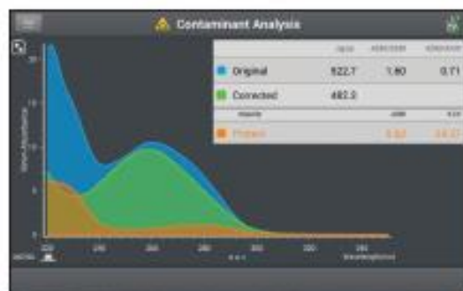
dsDNA sample contaminated with protein. The absorbance contribution from the protein (orange) is subtracted from the original result (blue) to obtain the corrected dsDNA concentration (green).
