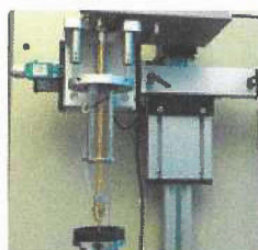
Mounting rack with extension line and sample cell, detailed view.
