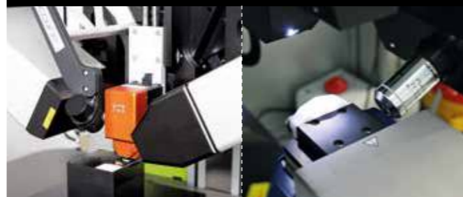
ep4 with adapted Nanosurf NaniteAFM QCM-D Quartz Crystal Microbalance from Q-Sense-Biolin integrated in the imaging ellipsometer
