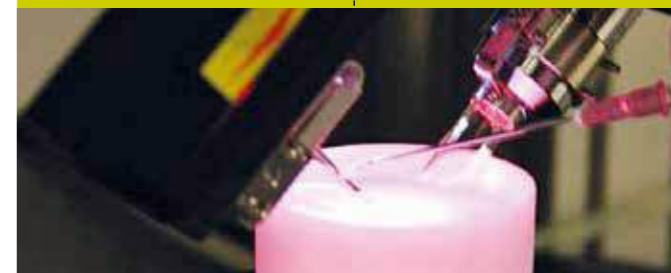
Light guide enables measurements at liquid/liquid interfaces and solid/liquid interfaces at variable angles between 40° and 72°
