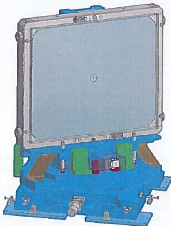
**Figure 3:** Assembly of the optomechanical mount G4. The three legs providing the three-axis rotation, equipped by flexure joints, are shown in dark yellow. The body of the mount is represented in dark blue, while brackets serving to fix the upper movable part during transport and installation are shown in green. The motorized stepper actuator serving for translational movement is seen in front near the mount base plate.
