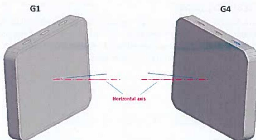
Figure 2: Spatial configuration of the gratings G1 and G4 in the L4 compressor: the gratings and their mounts are arranged symmetrically to each other. The gratings are oriented in space so that the front surface is rotated in yaw by 37.1 degrees with respect to the horizontal axis, and are inclined vertically (in pitch) by 4.07 degrees with respect to the horizontal axis. The required horizontal translation (see below) is in the direction of the horizontal axis.
