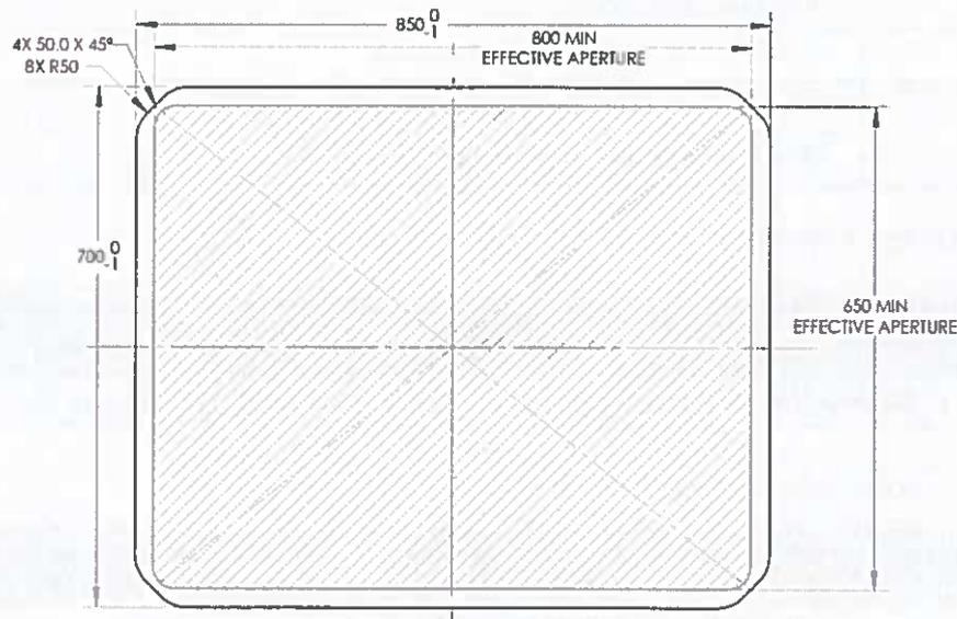
Figure 1: Dimensions of the diffraction gratings G1 and G4. The gratings are 100(+0/-1) mm thick.
