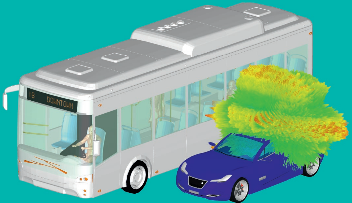
Installed performance: Radiation pattern for a V2V antenna on a car shadowed by a bus.
