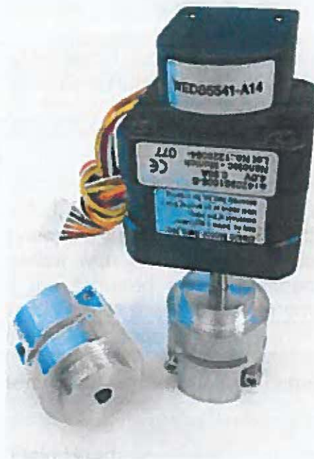
Figure 6: Exemplary stepper-Motor including encoder with D-cut and mechanical adapter with D-cut and mechanical joint to couple the stepper to one of the motion axis of the system. Please note – even though not drawn in the mechanical drawings all stepper motors will be outfitted with encoders as shown in this figure. The encoder is mounted on the extended motor axis that is shown in the mechanical drawings.
