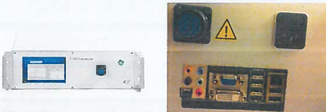
Figure 9: SGME®-controller with resistive touch screen SGME®-cable connector and power switch (Left). (Note, the cable connector can be also on the back side like shown on the right). Please note the Ethernet, 6 USB 2.0, VGA and DVI, mini-USB and Audio outputs. Note the layout will be changed to a more modern i7 embedded PC.
