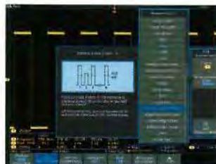
Each measurement has help text and graphics associated with it to help you understand the measurement's results.
