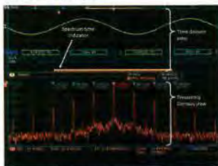
The orange bar in the MDO4000C Series always shows the Time Domain view of the analog and digital channels, while the lower half shows the Frequency Domain view of the spectrum analyzer channel. The orange bar in Spectrum Time is the view used to calculate the RF spectrum.
