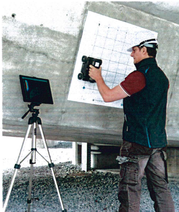
Proceq GPR Live performing an area scan with the aid of a Proceq grid paper
