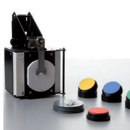
Integrating sphere for transmittance and diffuse reflectance measurements
