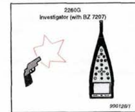
Fig. 13 Type 2260-G will measure reverberation time using just a starting pistol or other impulse sound source
