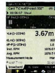
Fig. 2 Enhanced vibration allows velocity and displacement measurement
