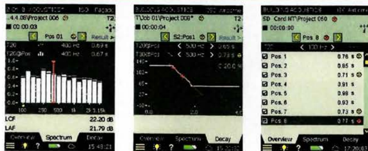
Fig. 8 Reverberation time spectrum (left); reverberation decay curve (centre); and overview of results (right)
