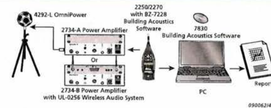
Fig. 2 Typical configuration for building acoustics measurements: sound source, amplifier, analyzer (including signal generator) and PC for reporting
