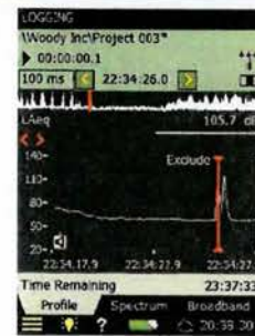
Fig. 9 Single-channel logging display showing a LAeq profile with marker functionality on the analyzer
