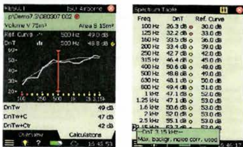
Fig. 9 With the required data measured, final results are shown, including the reference curve. For some results, the volume of the receiving room and the area of the partition must be entered
