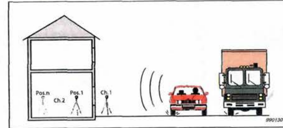
Fig. 11 Measuring sound pressure outside and inside the façade simultaneously - 2-channel measurement
