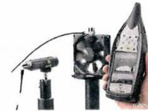
Fig. 10 Vibration measurement using a hand-held analyzer and Laser Tacho Probe Type 2981
