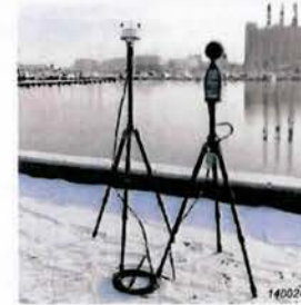
Fig. 15 Hand-held analyzer measuring outdoor noise using a weather station kit
