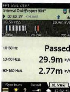
Fig. 5 The FFT Quality Check template provides specific customizable information for well-established tasks
