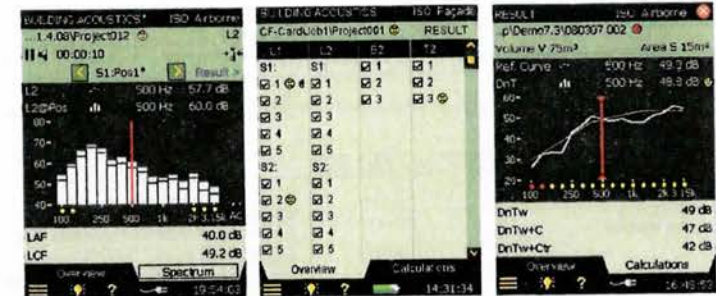
Fig. 25 Examples of building acoustic measurements using Type 2250/2270: L2 average and L2 at one position (Left) Overview of measurements (Centre) Final result (Right)
