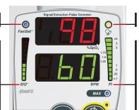
The Alarm Status Indicator flashes when an alarm condition is present.
